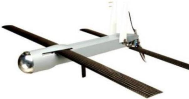
The UAV should weigh less than 36 pounds, and be launched from the aircraft and be able to fly for as long as 45 minutes at cruise speed; fly as fast as 90 knots; and be able to detect a target the size of a submarine.
