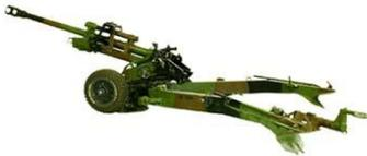
The LG 1 MARK II 105-MM HOWITZER is generally used to provide artillery fire support for light, highly mobile forces in Canada and abroad. Normally, it is pulled by a vehicle, such as a 2 ½ ton truck or a modified Grizzly. It can also be lifted by helicopter, dropped by parachute and transported by air. The LG1 is capable of engaging targets of up to 19 km away.
